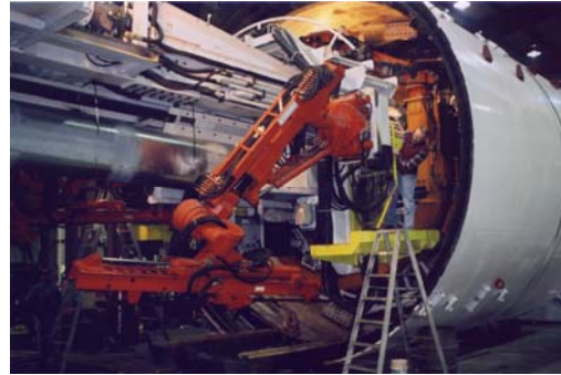
Traxxon fully articulating probing drill boom with SBH-15 positioners and 360° pedestal mounted on a tunnel boring machine.
