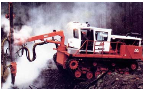
Drilling boom with SBH-15 swing and dump positioners mounted on a Traxxon tracked surface drill.
