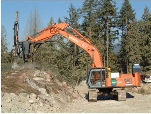
SBH-15 swing positioner mounted on a Traxxon excavator drill package.
